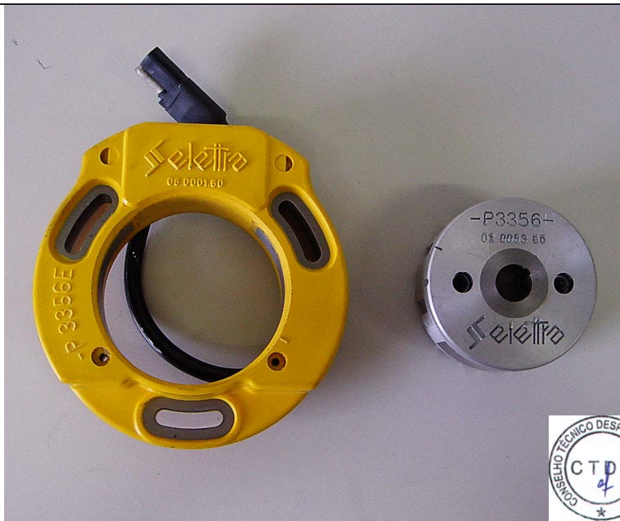
FOTO DO ESTATOR E DO ROTOR PHOTO OF THE STATOR AND OF THE ROTOR
